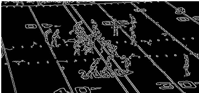
Fig. 3: Image following a canny edge detection
